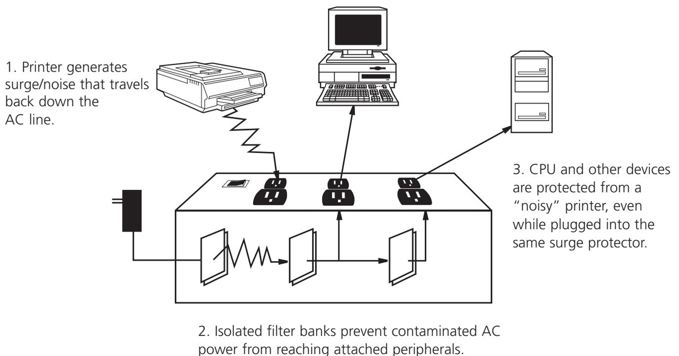
Fig. 5: Noise filters prevent AC-surge and line-noise contamination.
