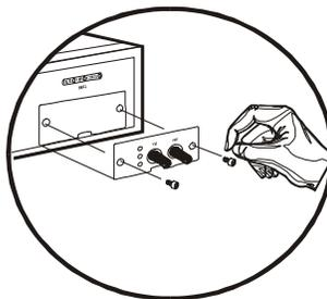
Figure 2: Removal of module cover plate
