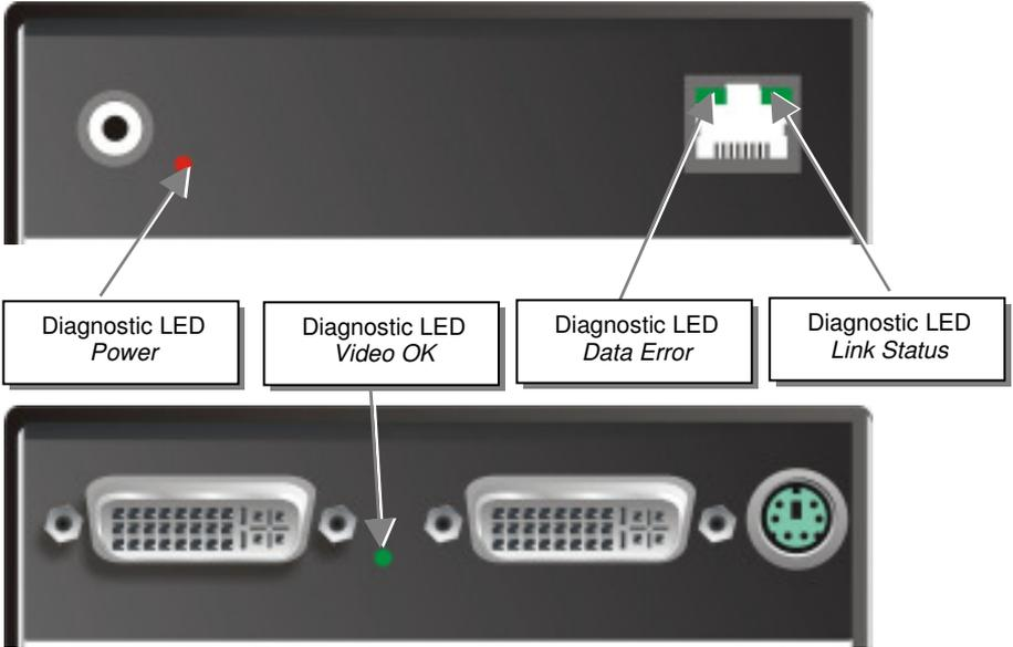
**Diagnostic - LEDs at DVI-D Cat X - Extender**
